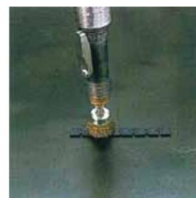
Deburring from formed resin parts
